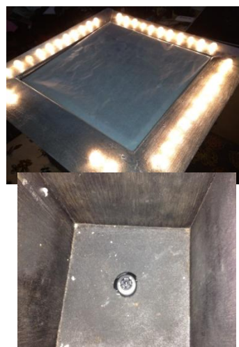
Fig. 3 Multi-touch table outside and inside view.
