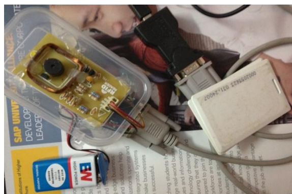
Fig. 8 RFID reader with RS 232 kit.
