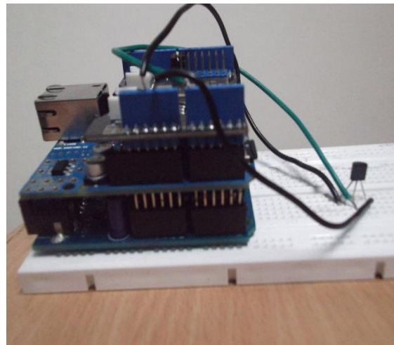
Fig. 2 : Ethernet shield and Bluetooth shield mounted over an Arduino and connected to LM35z temperature sensor
