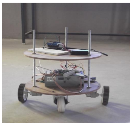
Fig. 5: Mobile robot with temperature sensing kit
