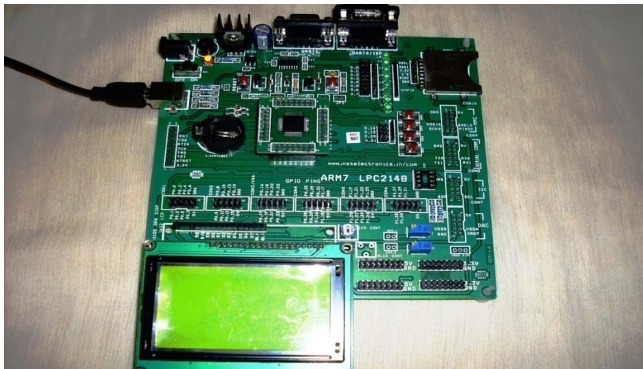
Fig. 8 : Hardware part with graphical LCD display
