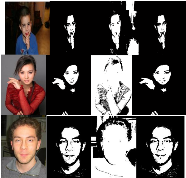
Figure 3. Column from left to right represents original images , Gaussian model’s result , Histogram result and Fusion approach’s result.
