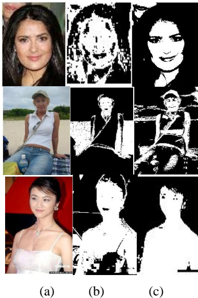
Figure 2. Comparison between CbCr and IBy space (a) Original Image. (b) CbCr Result and (c) IBy Result
