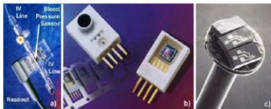
Figure (3) Disposable blood pressure sensor connected to an IV line (a), disposable blood pressure sensors (as shipped) (b), and (c) intracardiac catheter-tip sensors for monitoring blood pressure during cardiac catheterisation, shown on the head of a pin.
