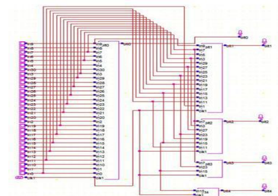
Fig.13. Schematic view of 5-bit dynamic thermometer encoder for flash ADC.
