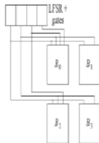
Figure 3.4 Hardware implementation of the test process for the FIFO buffers. (b) Implementation of test circuit.
