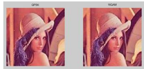
Fig.6. Received image using QPSK and 16-QAM for SNR=15
