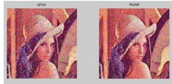
Fig.5. Received image using QPSK and 16-QAM for SNR=10
