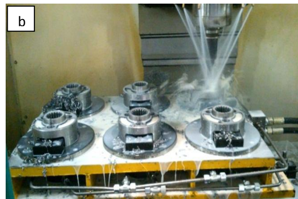
Fig 2.5.1.b. Machining using Fixture
