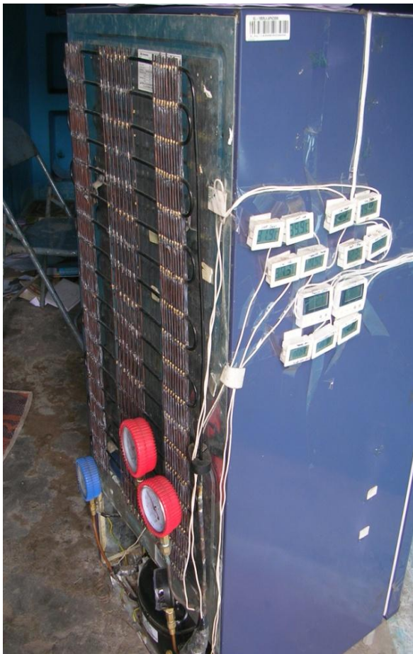
Fig. 1. Finned tube condenser used for experimental study
