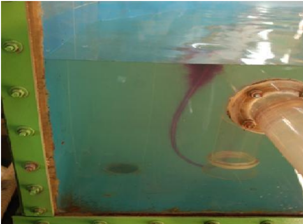
Fig. 19 Photographic view showing position of vortex when water level reduces below MDDL
