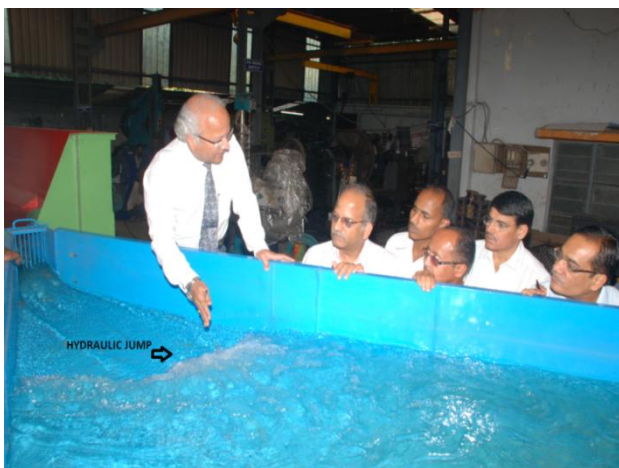
Fig. 7 Photographic view showing hydraulic jump
