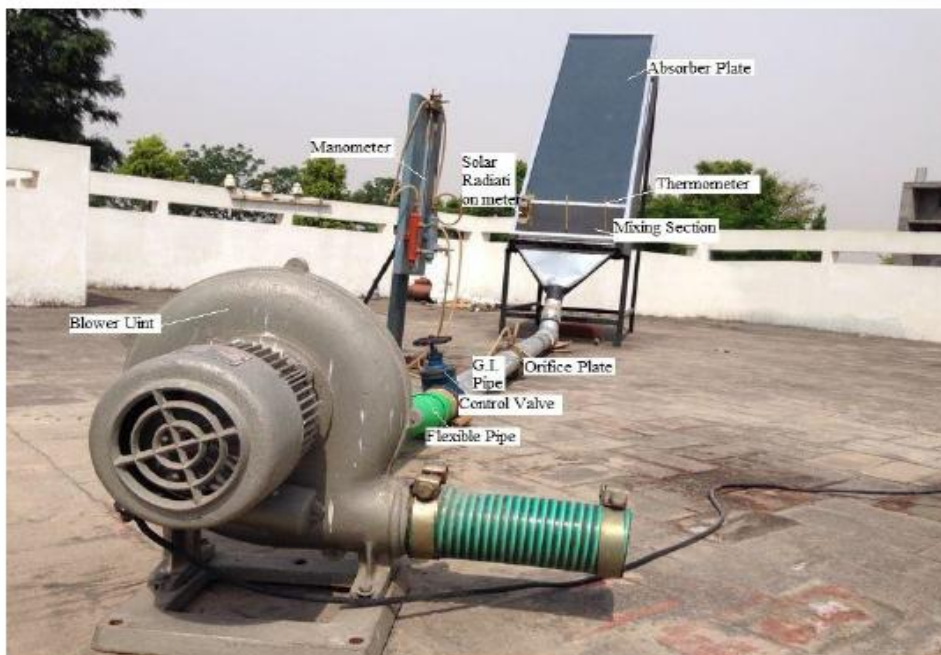
Figure 2 Direct photograph of the experimental setup.
