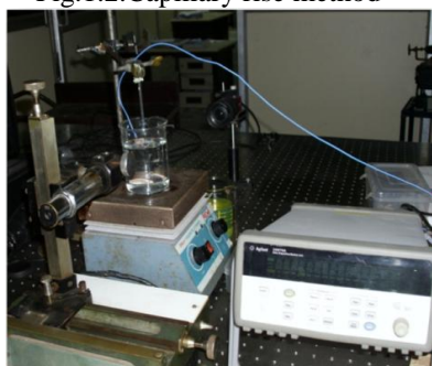
Fig.1.3.Travelling microscope for capillary rise measurement
