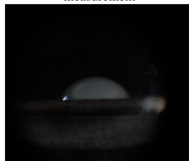
Fig.1.7. Image of 0.01% \text{Al}_2\text{O}_3 Nanofluid angle droplet on copper plate
