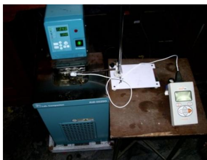
Fig.1.8. Setup for thermal conductivity measurement
