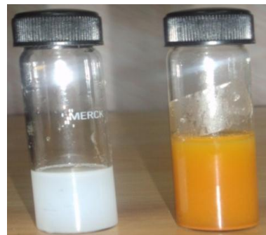
Fig.1.35. 0.05% vol Al 2 O 3 nanofluid before and after the operation of heat pipe.
