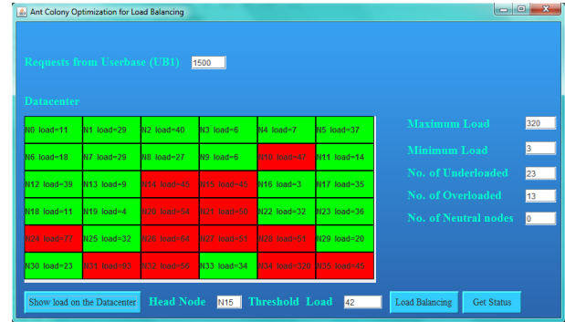
Figure I. Simulation: Load on simulated servers without Load Balancing Technique
