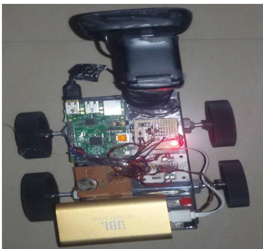
Fig: Hardware section of Robot
