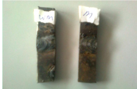
Fig 6: Welding specimens for impact test
