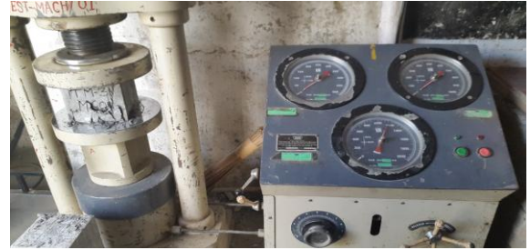
Fig.6. Compression Test on cube without silica fume & glass fibre
