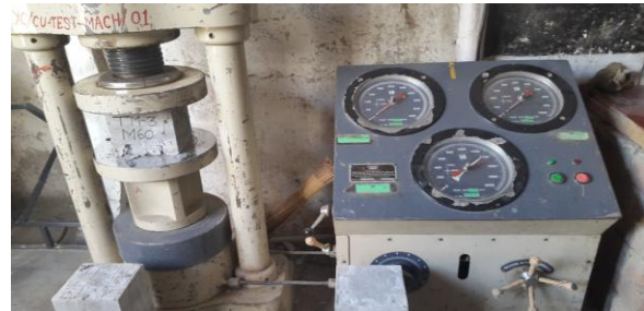
Fig.7. Compression test on cube with silica fume & glass fibre
