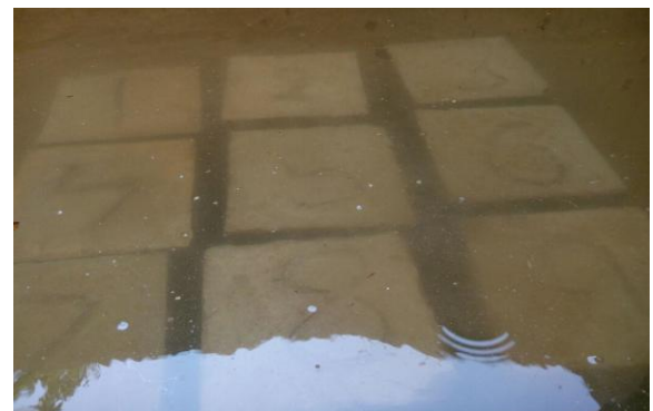
Fig.4. Curing of Cubes
