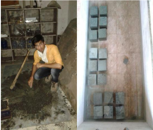
Figure 2: Casting of Concrete Cubes
