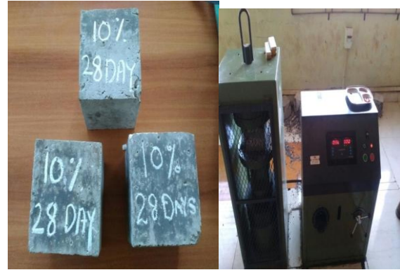
Figure 3: Testing of Concrete Cubes
