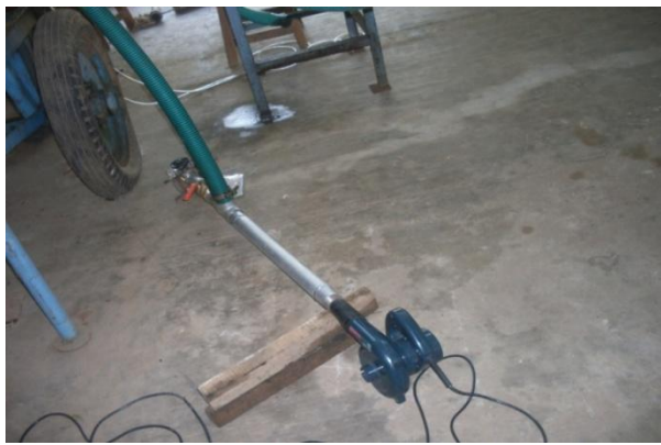
Fig 4.2: Blower used for forced flow experimentation
