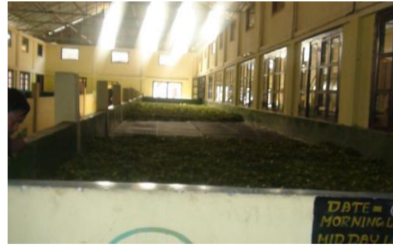
Fig.3: Withering Trough of Rijo Tea Plant
