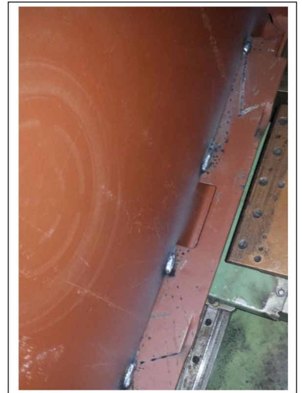
Figure 8: Uniform welding beads obtained by welding Robot on Joint strip of Defender Safe.
