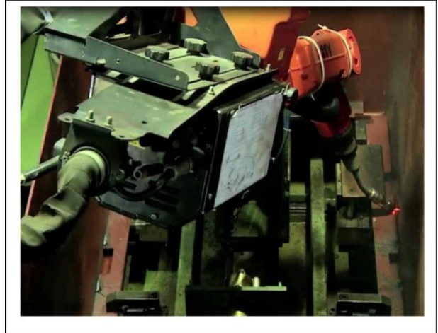
Figure 7: Robot Welding Class-A Body of Defender Safe
