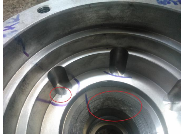
Fig. 2: Casting with Shrinkage Cavities and Sand Drop Defect
