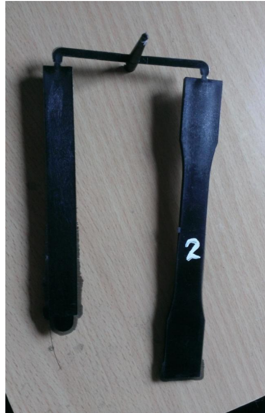
Specimen made for Tensile and flexural test
