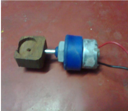
Figure 3 Stepper Motor connected with Neodymium Magnet
