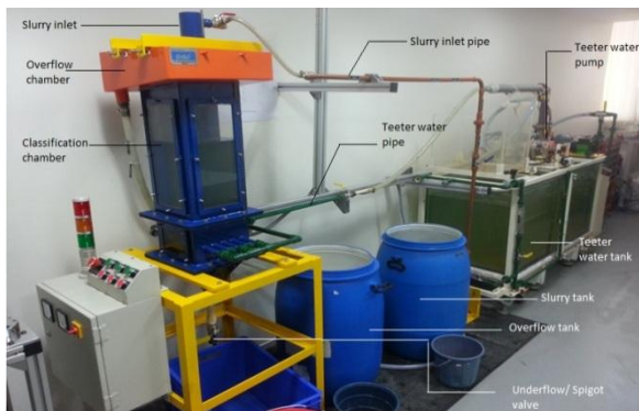
Fig.1. Conical base classifier test setup
