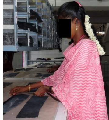
Figure 6. Fusing operation done by the workers
