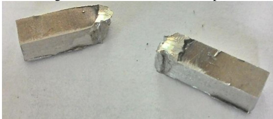
Fig. 5. Broken Impact Test Samples
