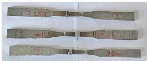
Fig. 4. Broken Tensile Test Samples
