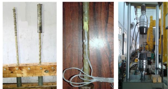
Figure 2: GFRP rebar capping; GFRP rebar with strain gauge; Testing machine
