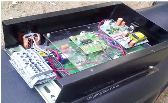
Fig: 7 Motor controller used in the car
