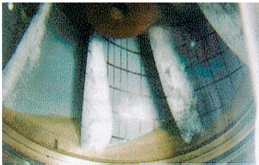
Fig. 14. Leading edge cavitation at inlet of pump
