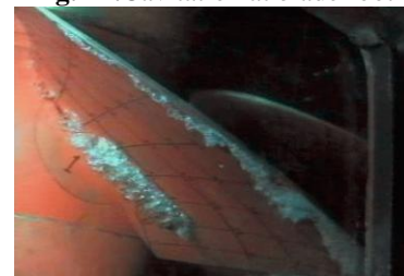
Fig. 13. Cavitation at blade tip
