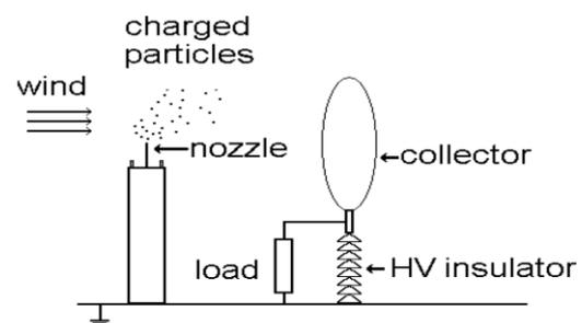
Fig2. Type A implementation of the EWICON system with an insulated collector.
