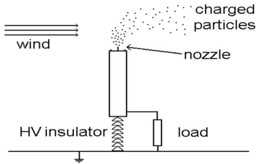
Fig3. Type B implementation of the EWICON system without collector.
