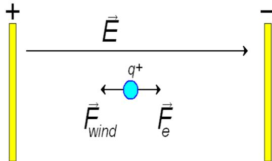
Fig1. A positively charged particle is pushed towards the positive electrode by the wind against the direction of electric field.
