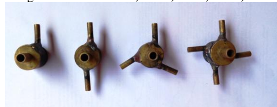
Fig. 3: Inlet nozzles used for experimentation
