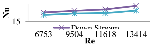
Fig. 12 Variations in Nusselt number with Reynolds Number with various pulsation Frequencies at 100 W
