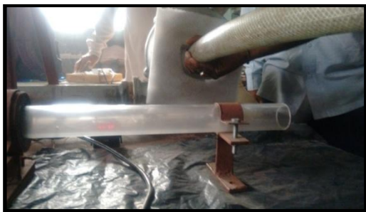
Fig. 18 Flow pattern for pulsation frequency f = 1.67 & Re = 6753
