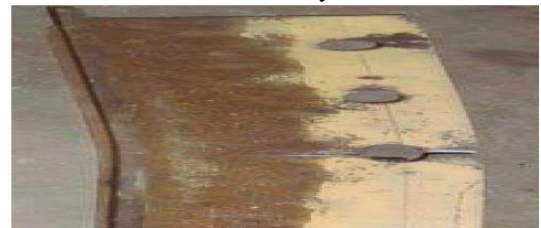
Fig. 4.2 Partial net section ruptures, with large eccentricity
