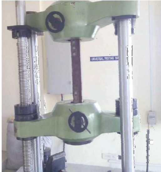
Fig. 3.1 Specimen grip assembly in UTM
