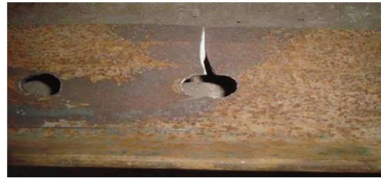
Fig. 4.1 Partial net section ruptures, with small eccentricity
