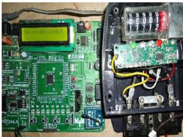
Fig.4: Electric meter interfaces with Microcontroller showing Unit count and Bill amount
